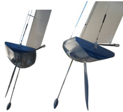
Fig. 6. Sailboat model applying bending rudder device
