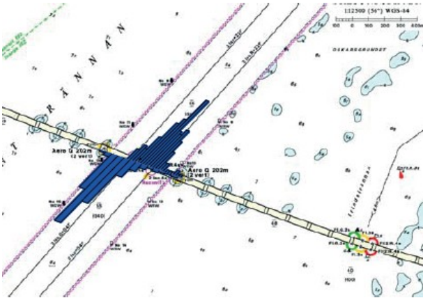
Fig. 1. Navigational conditions in the vicinity of the Øresund bridge with ship traffic distribution (passenger vessel, winter months)
