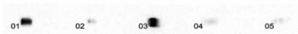
Fig. 7. Photos of laser spots of heads 01–05. Uniform scale of photos was maintained. Negative picture. Photos were taken in non-reflection chamber on the distance of 20 metres with flow of external light below 0.001 lx. Exposure time: 15 s
