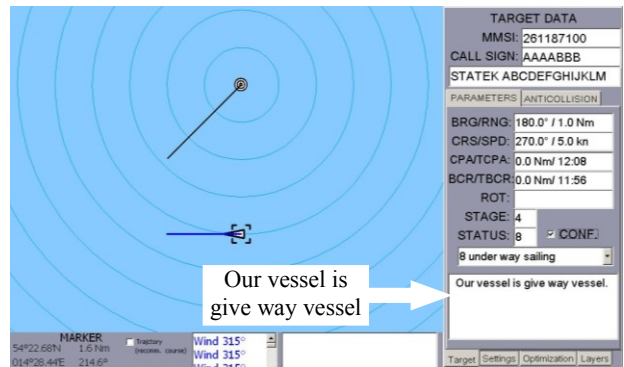
Rys. 6. Qualification of the encounter according to the COLREGs
