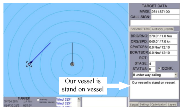
Fig. 1. Qualification of the encounter according to the COLREGS
