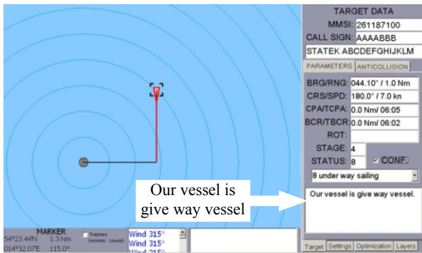
Fig. 3. Qualification of the encounter according to the COLREGs
