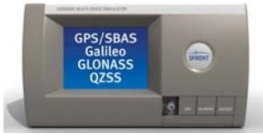
Fig. 4. Multi-GNSS Spirent GSS8000 simulator (frequencies – GPS: L1, L2, L5; Galileo: E1, E5ab, E6; GLONASS: L1, L2; SBAS: L1, L5) (picture SPIRENT)
