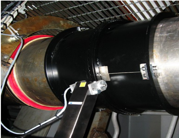
Photo 1. Toothed rings and laser sensor ETNP-8 mounted at intermediate shaft
