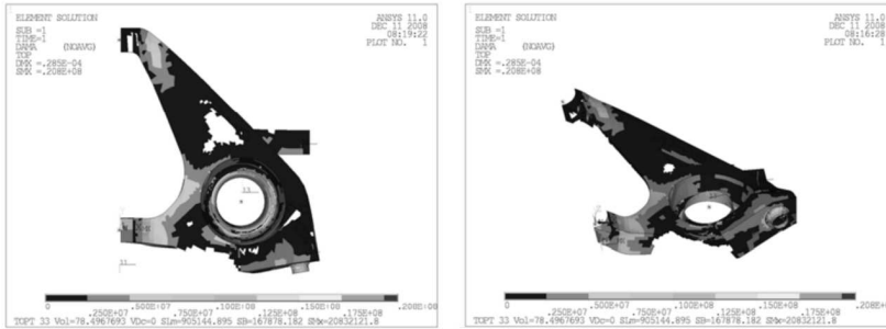
Fig. 7. Results of topology optimization of the second stage of optimization; objective function f(\eta) = 4484.54 \text{ g}
