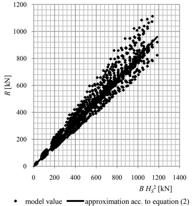
Fig. 6. Significant values of added resistance on bow wave  $R$  calculated by means of accurate numerical methods and equation (2),  $B = \text{var}$ ,  $H_S = \text{var}$ , wave spectrum – JONSWAP, vessel speed  $v = 10 \text{ m/s}$
