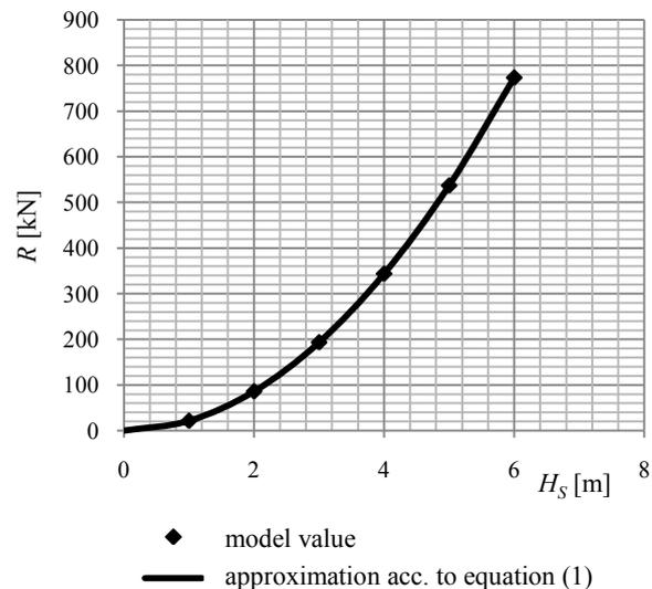
Fig. 2. Significant values of added resistance in bow waves  $R$  calculated by means of accurate numerical methods and equation (1),  $H_S = \text{var}$ ,  $C_M = 0.97$ ,  $B = 27.14$  m, wave spectrum – JONSWAP, vessel speed  $v = 10$  m/s
