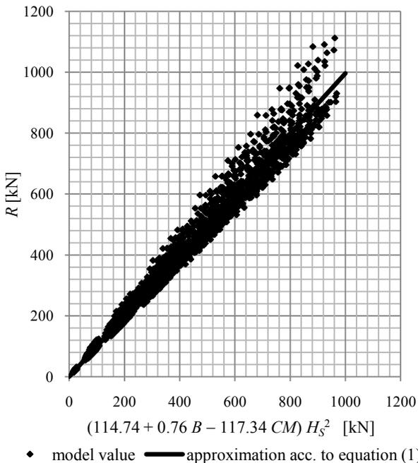
Fig. 5. Significant values of added resistance in bow waves  $R$  calculated by means of accurate numerical methods and equation (1),  $B = \text{var}$ ,  $CM = \text{var}$ ,  $H_S = \text{var}$ , wave spectrum – JONSWAP, vessel speed  $v = 10 \text{ m/s}$
