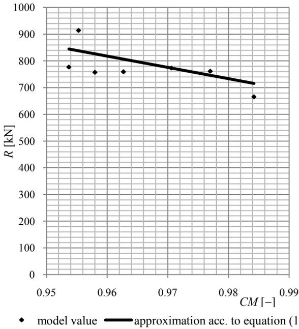
Fig. 4. Significant values of added resistance in bow waves  $R$  calculated by means of accurate numerical methods and equation (1),  $CM = \text{var}$ ,  $B = 27.1 \text{ m}$ ,  $H_S = 6 \text{ m}$ , wave spectrum – JONSWAP, vessel speed  $v = 10 \text{ m/s}$
