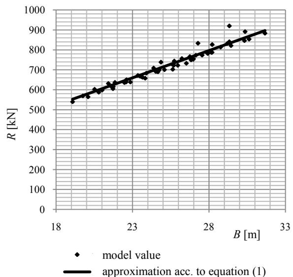
Fig. 3. Significant values of added resistance in bow waves  $R$  calculated by means of accurate numerical methods and equation (1),  $B = \text{var}$ ,  $C_M = 0.97$ ,  $H_S = 6$  m, wave spectrum – JONSWAP, vessel speed  $v = 10$  m/s
