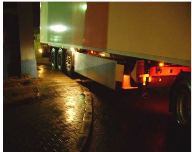
Fig. 7. The area on the side of the road illuminated by the extra trailer lights when cornering
