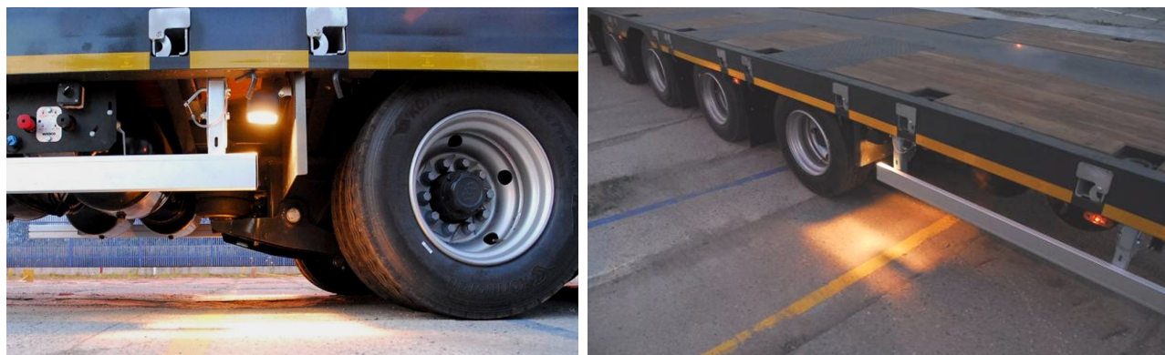
Fig. 9. View of the lamp and its mounting on a Wielton trailer for transporting oversized cargo and the area around the wheels lit up by the extra lamp
