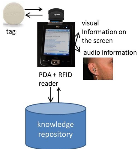
Fig. 3. The way of sharing information using RFID technologies
