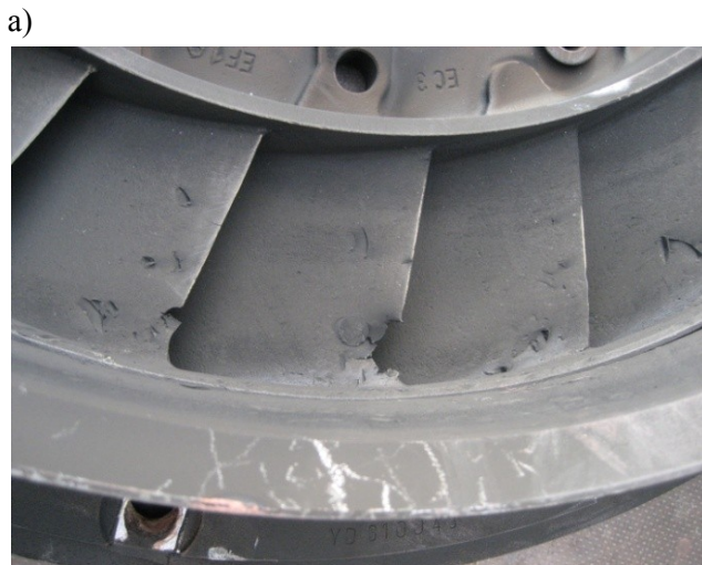
Fig. 10. Results of the random damage to the VTR-454-11 turbocharger; a) damage to turbine guide vane / stator blades due to a broken or torn injector pin, b) the damaged labyrinth sealing due to the shortage of an air barrier
