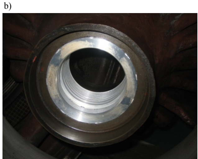
Fig. 10. Results of the random damage to the VTR-454-11 turbocharger; a) damage to turbine guide vane / stator blades due to a broken or torn injector pin, b) the damaged labyrinth sealing due to the shortage of an air barrier
