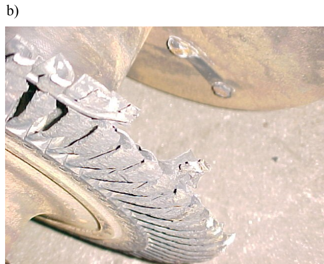
Fig. 11. Results of the random damage to the ABB VTR-250 turbocharger [13]; a) damage to the compressor rotor caused by the seizure of the bearings of the VTR-250 turbocharger, b) damage to the turbine rotor by a foreign body – the ABB VTR – 250 type turbocharger
