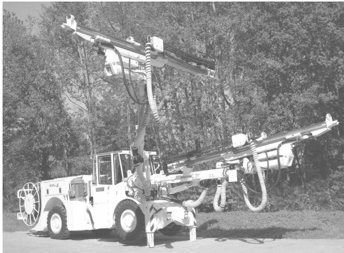
Fig. 10. Mining machine Face Master 2.5 with two booms installed ( www.minemaster.eu [13])
