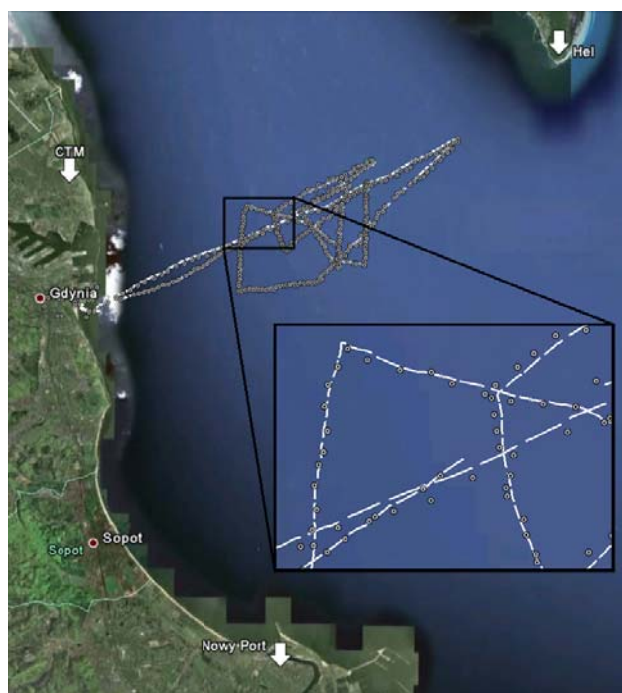
Fig. 4. Deployment of ground stations (arrows) and a path of GPS and GLONASS positions (dotted line) and readings of autonomous AEGIR system (dots)
