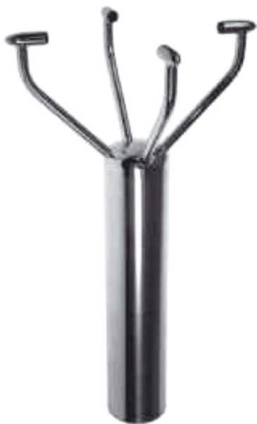
Fig. 17. The WINDOBSERVER II anemometer antenna [12]
