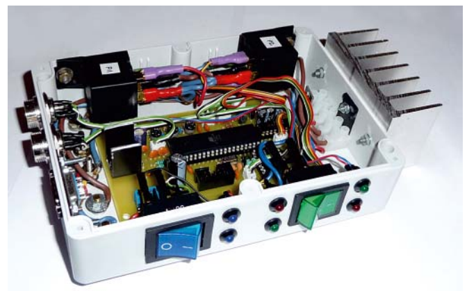
Fig. 10. Electronic elements for tunnel thrusters drive
