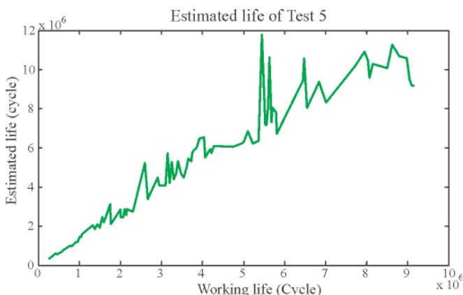
Fig. 5. Estimated life of the ball bearing in Test 5 (defect in outer race)
