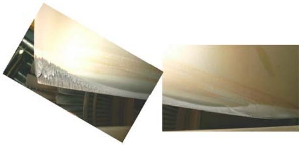
Fig.15 Photos of inlet edge erosion of the blade of the last rotor stage after 40 000 h service, acc. [16].
