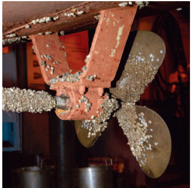
Fig. 2. Cantilever open bearing of yacht's propeller shaft
