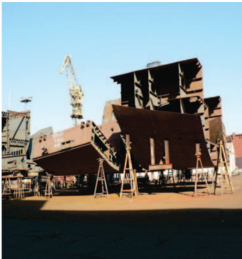
Fig. 2. Prefabricated ship's hull units and blocks in positions in which they are measured
