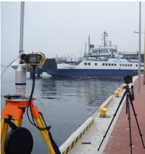
Fig. 4. Measurement bench (in the foreground rangefinder MDL in the background ferry “Bielik”)
