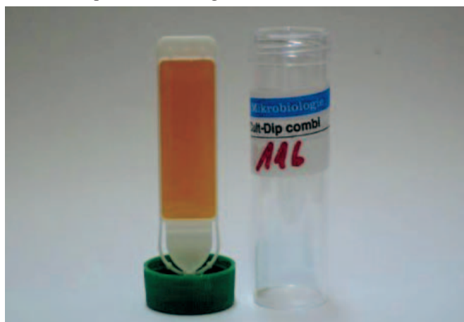
Fig. 2. Plastic paddle coated with nutrient (prod. Merck) used in dip-slide method
