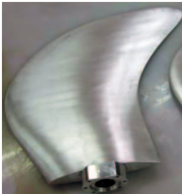
Fig. 1. The model of the hydrofoil N manufactured in aluminum alloy using the numerically controlled milling machine
