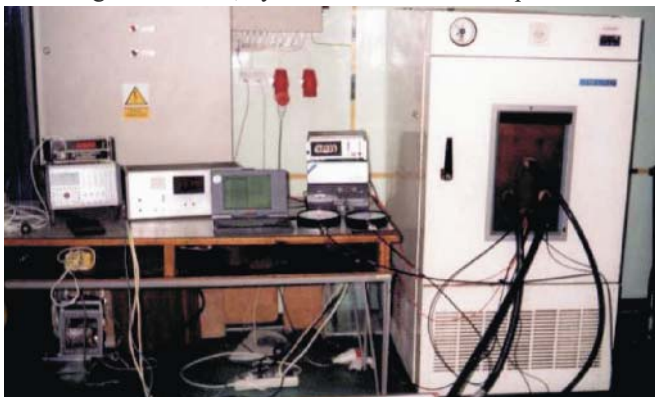
Fig. 7. Low-temperature chamber and measuring system installed in the laboratory of the Chair of Hydraulics and Pneumatics
