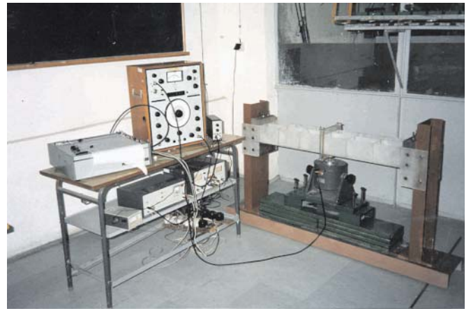
Photo 2. The tested model connected with vibration exciter
