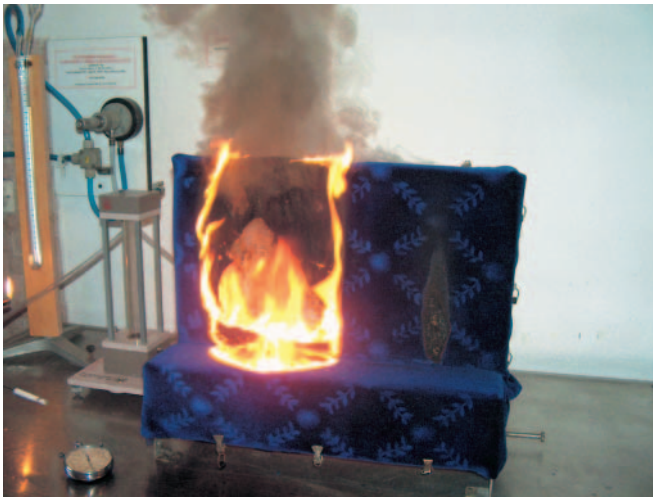
Fig. 3. Inflammability tests of upholstery furniture according to IMO FTP Code, Part 8 (test of torch flame equivalent to that of burning match) [4]; exposure time to flame action equal to 30s.
