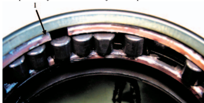
Fig. 8. Damaged central bearing, earlier diagnosed using the FAM-C method: 1 – broken cage separator ring
