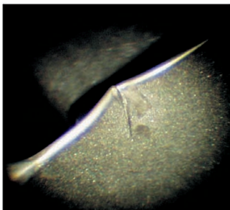
9th stage of compressor of LM-2500 engine – dent and crack at the edge of attack of rotor blade
