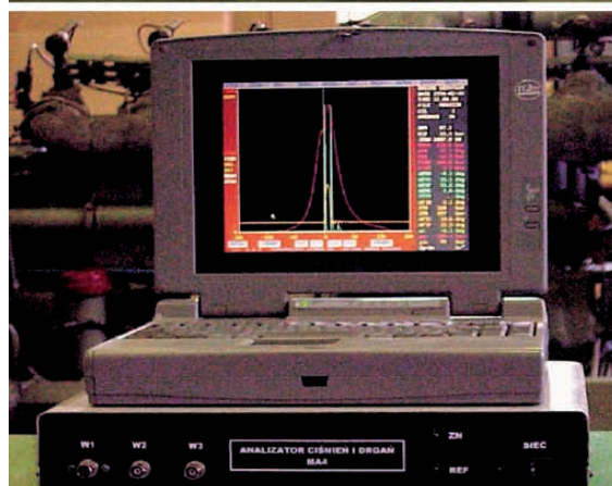
Fig. 1. The diagnostic team of Dr Polanowski at the stand for testing the cylinder systems of Henschel engines – cylinder pressure analyzer; example results of testing the engine combustion chamber
