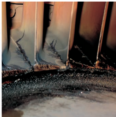
6th stage of propulsion turbine of LM-2500 engine – traces of carbon deposit on rotor blade surface
