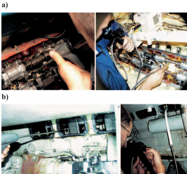
Fig. 6. Ways of inserting the end of borescope and fiberscope into cylinder interior of : a) M401A-1 diesel engine – through the holes remaining from dismantled injectors, b) 16V149TI Detroit Diesel engine – through inlet air windows in cylinder liner .
