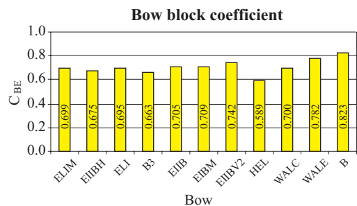
Fig. 6. The bow block coefficient C_{BE} (the bows are ranked on the basis of their hull resistance values at the water depth of 3.4 m, see Fig.4) .
