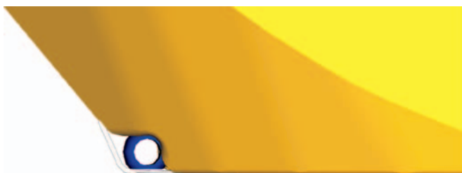
Fig. 2. Side view of the hull. The propulsion unit with the screw propeller of 400 mm diameter .
