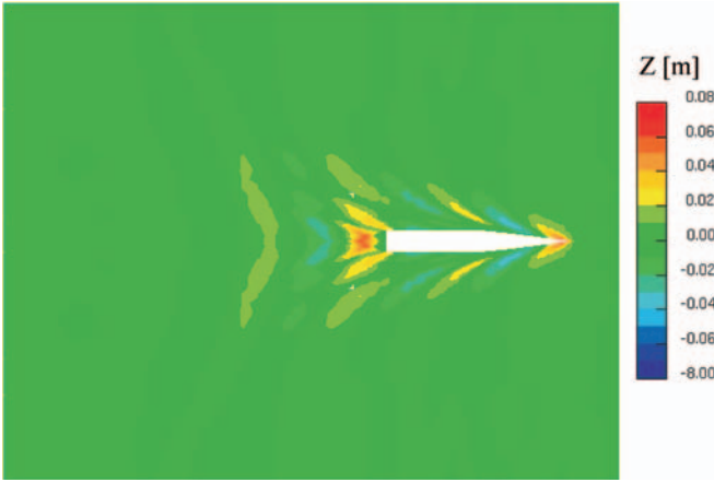
Fig. 16. Wave contour at Froude number F_n = 0.3 .
