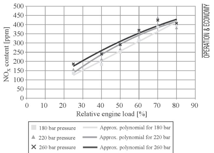
**Fig.1.** NO<sub>x</sub> content in exhaust gas in function of three different injector opening pressures
