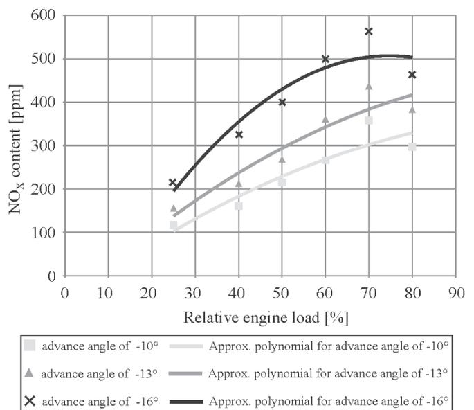
**Fig.2.** NO<sub>x</sub> content in exhaust gas in function of three different advance angles of fuel injection
