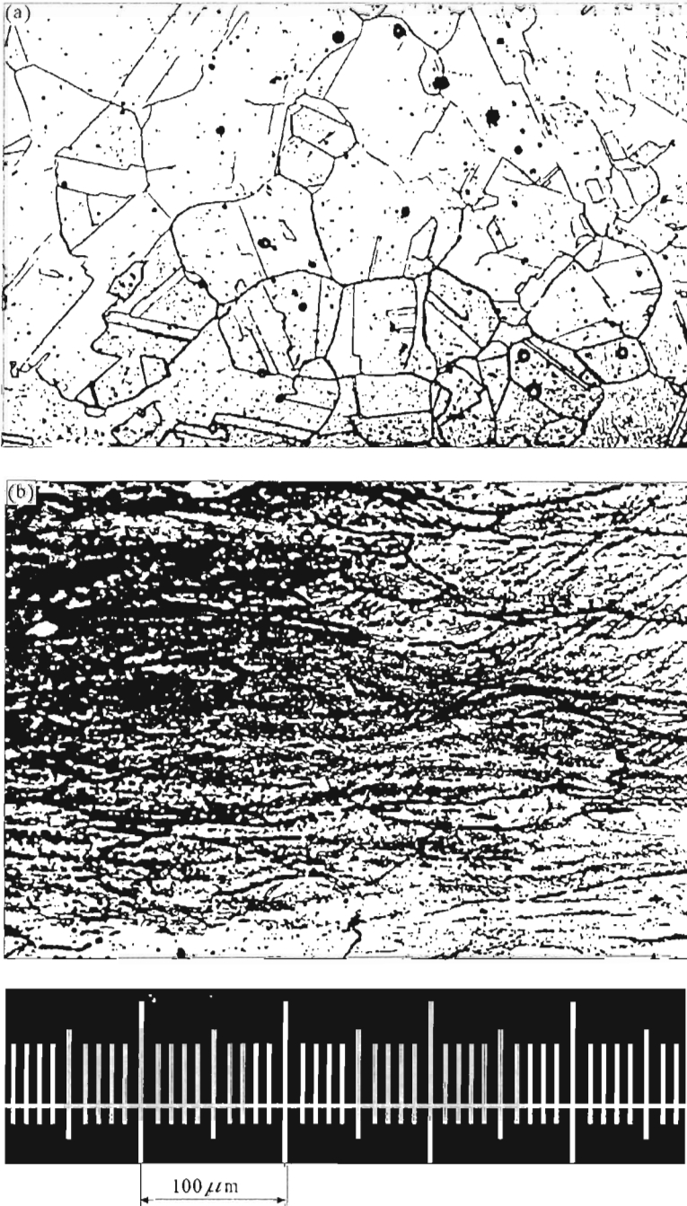
Fig. 1. Optical micrograph of samples of stainless steel surface before straining: (a) – after heating, (b) – after rolling
