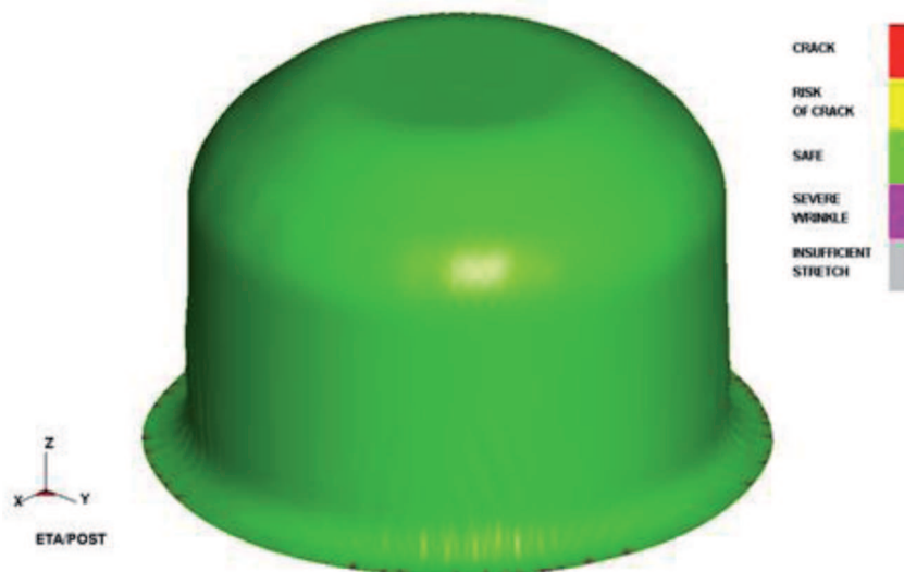
Fig. 10. Final shape of bearing housing
