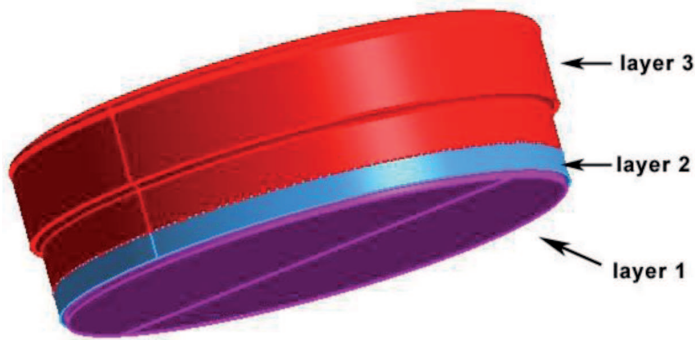
Fig. 4. Three-layer rubber pad model
