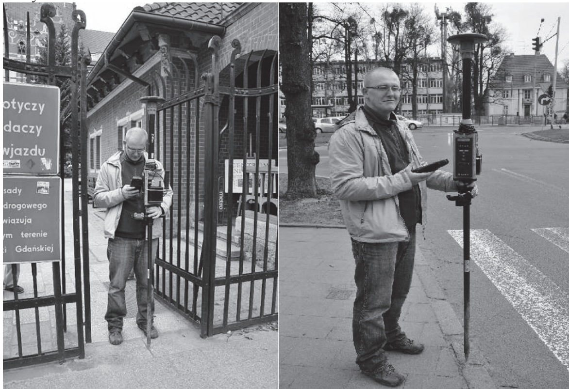
Fig.4. Precise data acquisition with geodetic DGPS receiver.
