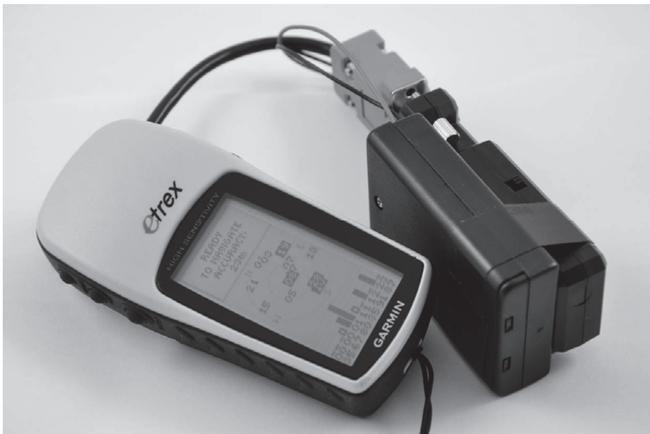
Fig.3. External DGPS receiver connected to the Bluetooth adapter.
