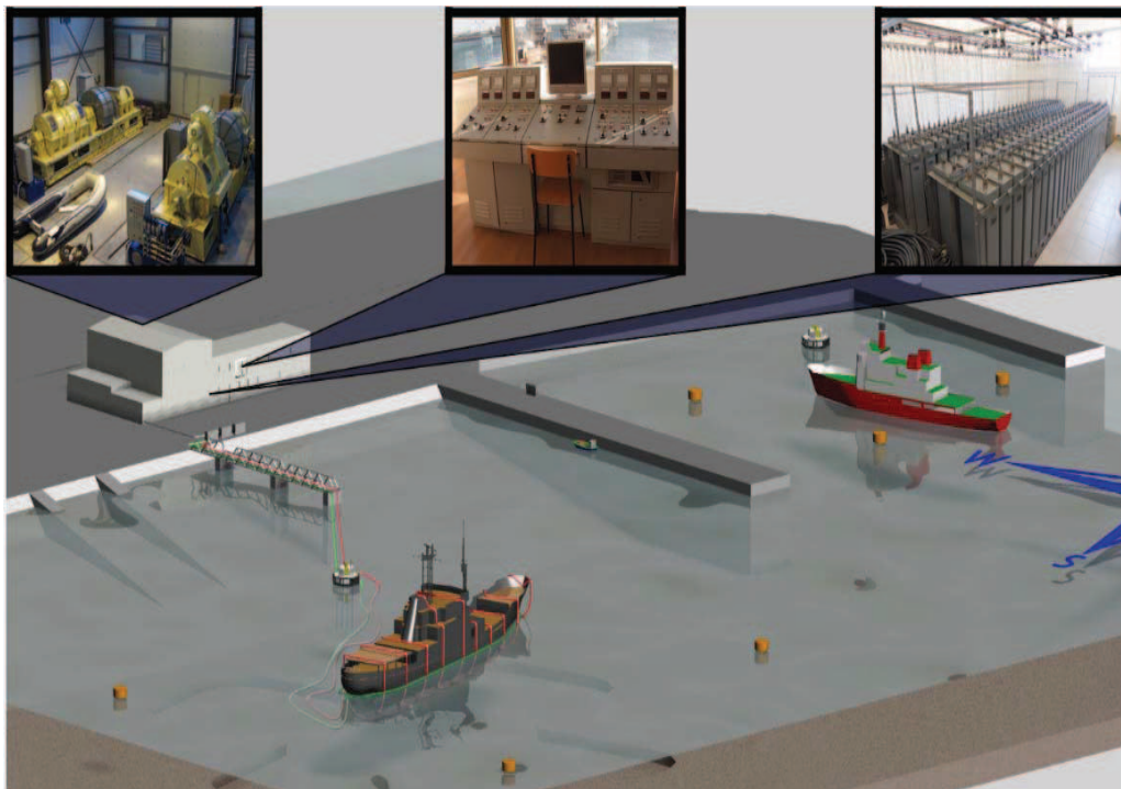
Fig.10. The control building, magnetic range equipment and treatment facilities. The ship is rigged with X-solenoid (red) and Z-loop (green) in deperming process.
