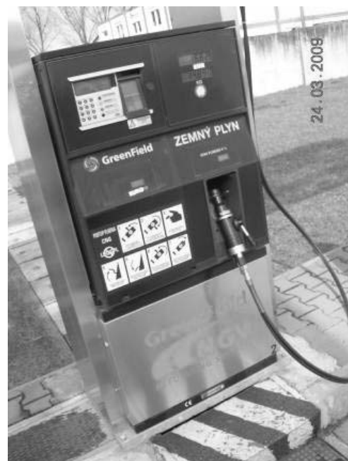
Fig. 1. CNG dispensers - Greenfield A.G.
