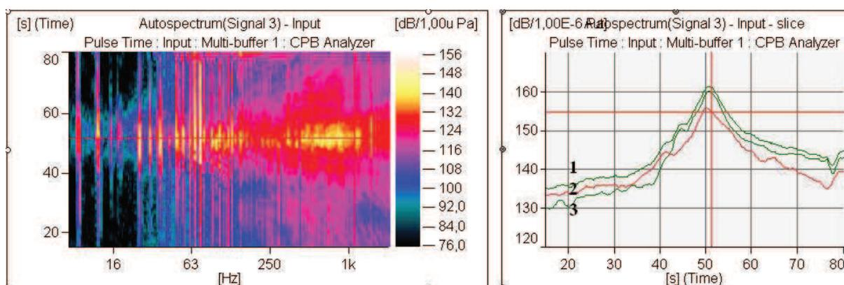
Fig.5. Noises of the right ship's motor registered at the speed  $v = 9$  [kt]. Hydroacoustics pressure level 1 – ship, 2 – ship's propeller, 3 – driving system
