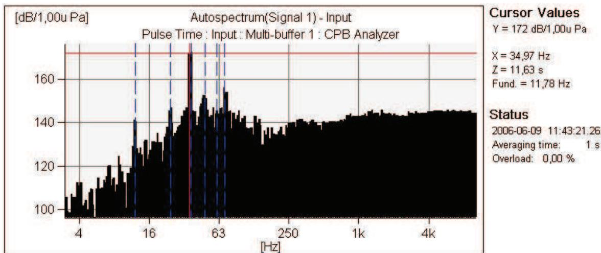
Fig.2. Spectrum of the hydroacoustics noise obtained from spectrogram presented on fig.1
