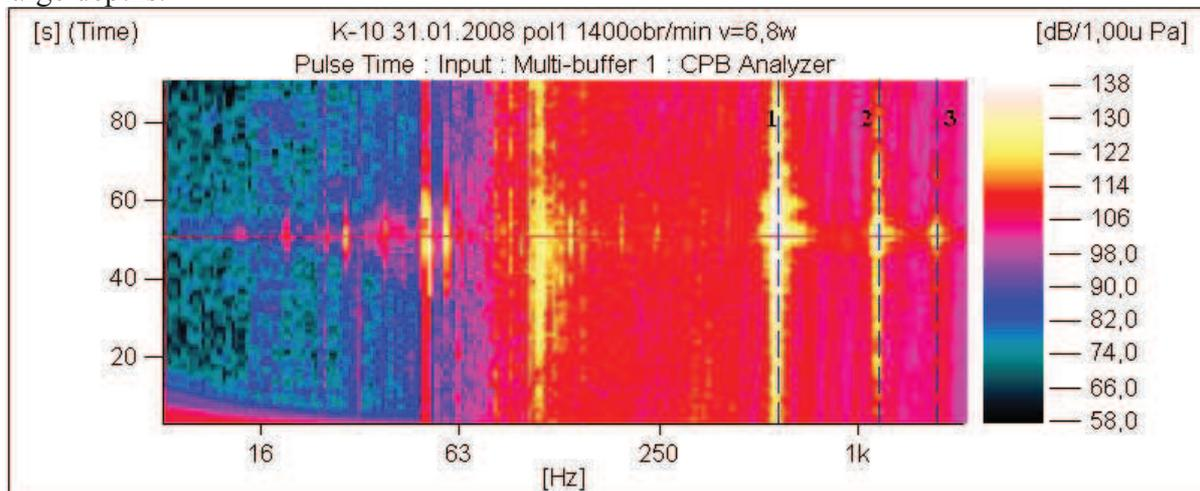
Fig.3. Spectrogram of the hydroacoustic noise where: 1 – the basic frequency associated with the ship's propeller; 2 – its II harmonic; 3 – its III harmonic
