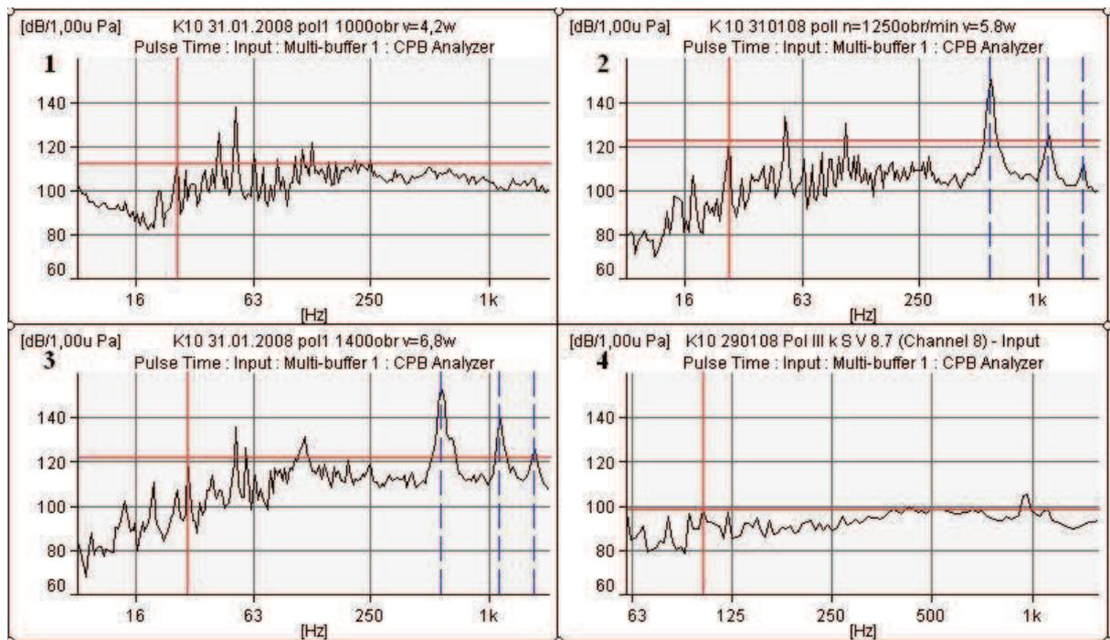
Fig.4. Spectrum of the hydroacoustics noise where: 1. registered at the speed  $V= 4.2$  [kt], 2. registered at the speed of  $V= 5.8$  [kt], 3. registered at the speed of  $V= 6.8$  [kt], 4. registered at the speed of  $V= 8.7$  [kt]
