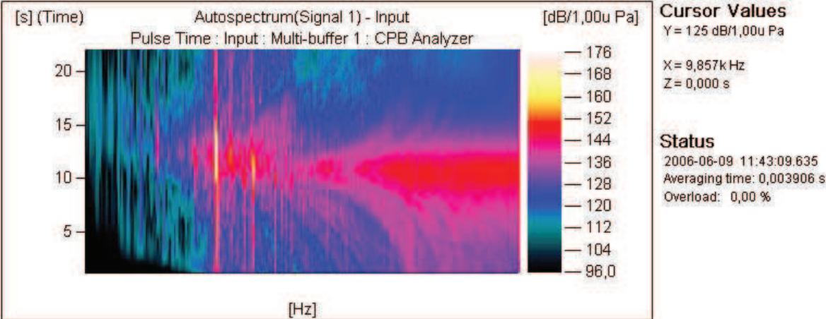
Fig.1. Spectrogram of underwater noise of the cutter at V >30 [kt]
