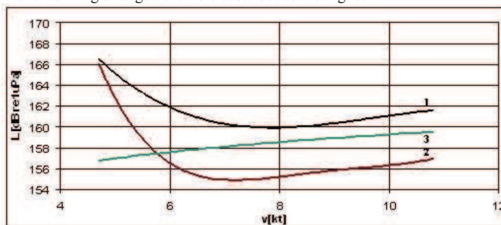
Fig.6. Dependences of noise levels in the function of the ship's speed where: 1 – ship, 2 – cavitation of ship's propeller, 3 – driving system
