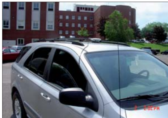
Fig. 2. The rover antenna mounting
