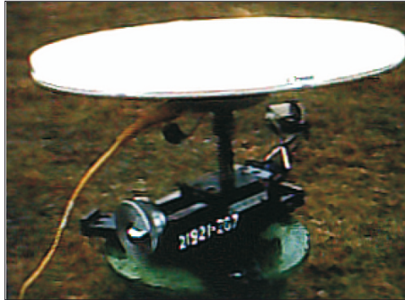
Fig. 5. Photo of the micrometrical device with mounted GPS antenna on it in the process of metrological control of the GPS complex
