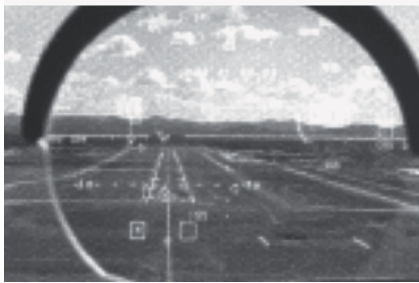
Fig. 8. Landing safety systems projected at cockpit HUD: a) Honeywell Corp. designed for Gulfstream [17]; b) Flight Dynamics simulator for pilot training [18]
