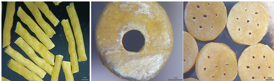
Fig. 3. Examples of real shapes of analysed fine-grained, tube propellant B (on the left), tube propellant C (in the middle) and 7-hole propellant D (on the right)
