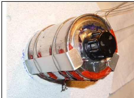
Fig. 3. View of the battery BTR-03 with mounted coated thermocouples which are used to measure the temperature on the outer surface of the battery cup
