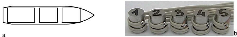
Fig. 5. Samples for compression tests: a – the shape and way of samples preparation, b – the samples with the stuck on strain rosettes, ready to tests
