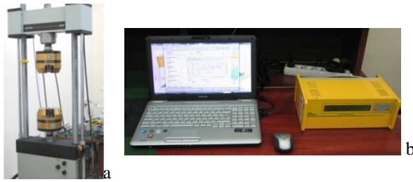
Fig. 2. Static compression test stand: a – Instron 8802 material testing machine, b – extensometric testing equipment to strain measurement
