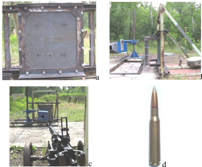
Fig. 4. The frame to fix the Armox 500T plates (a), DP testing stand (b), DSZK rifle (c), 12.7 mm cartridge with the B-32 type API projectile (d)
