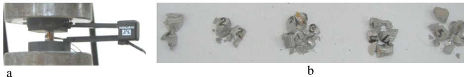
Fig. 6. Samples for compression tests: a – in jaws of the mechanical testing machine, b – after tests
