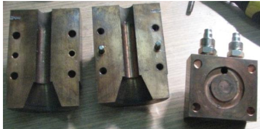
Fig. 5. Mould for bar casting of 10 mm diameter and 50 mm length
