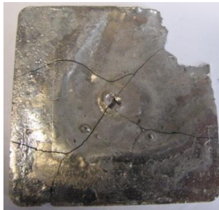
Fig. 8. Plate of 5 mm thickness cast from master alloy no 2
