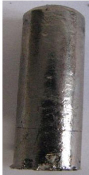
Fig. 7. Bar of 10 mm diameters cast from master alloy no 2
