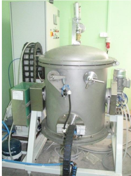
Fig. 4. Stand for melting and pressure die casting of amorphous alloys (left and front view)
