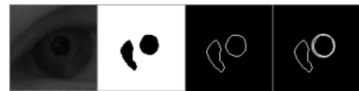
Fig. 7. Example image of the eye in half-extreme position and the successful circumscribed circle on the one of the two contours found in the ROI with two black-coloured objects.
