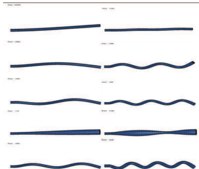
Fig. 3. Eigenmodes for cylindrical barrel (from the left side to the right side is from 1 to 10 respectively)
