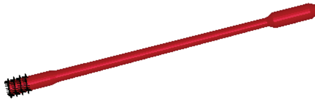
Fig. 2. Design of the 7.62 mm barrel with a muzzle compensator and fixed end around the chamber at the length of 26 mm
