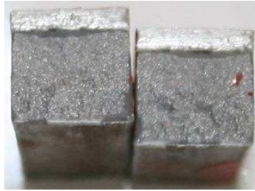
Fig. 4. Fracture surface of tested material C30E in the supplied state
