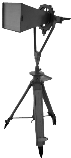
Fig. 4. TEM horn antenna II6-23 (transmitting antenna in microwave imaging system).
