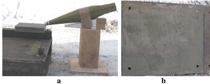
Fig. 4. Panel 1 with the ERAWA-1 cassette before the initiation of the PG-7 projectile at an angle of \alpha = 72^\circ (a) and the RHA 2 plate (witness) after the initiation of the projectile (b)
