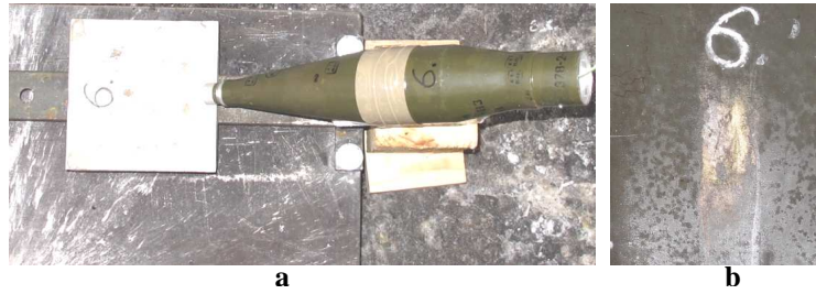
Fig. 10. Panel 6 with the ERAWA-1 cassette before the initiation of the PG-7 projectile at an angle of \alpha = 60^\circ (a) and the RHA plate 2 (witness) after the initiation of the projectile (b)
