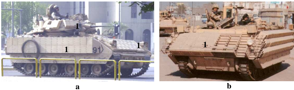
Fig. 1. Light fighting vehicles with ERA cassettes (1) protecting from PG-7 type shaped charge projectiles; a – Bradley with different non modular cassettes, b – FV432 Mk3 BULLDOG with modular cassettes
