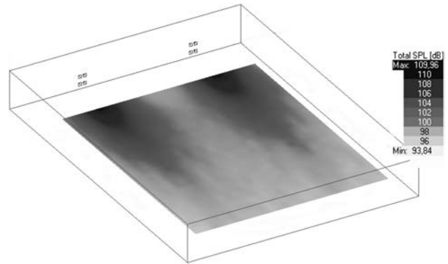
Fig. 5. SPL parameter distribution for the Community central sound system.
