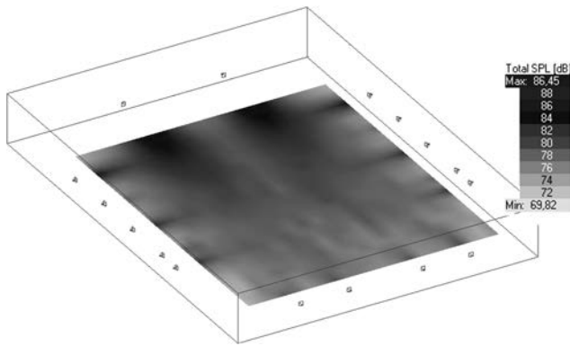
Fig. 8. Distribution of the SPL parameter in the reinforced area for the multi-channel system for sound creation in open areas.
